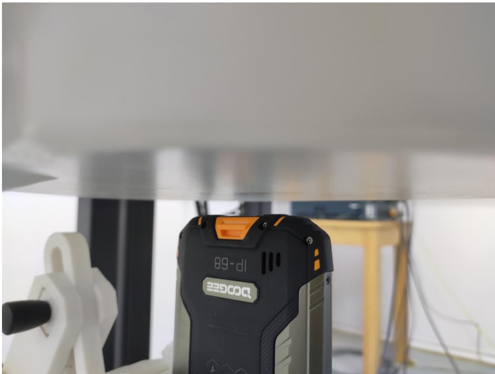
10mm body-worn Bottom Side Setup Photo (hotspot)
