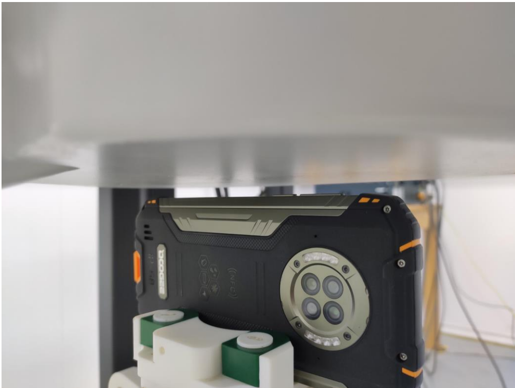
10mm body-worn Right Side Setup Photo (hotspot)
