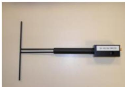
Figure 1 – Satimo COMOSAR Validation Dipole
