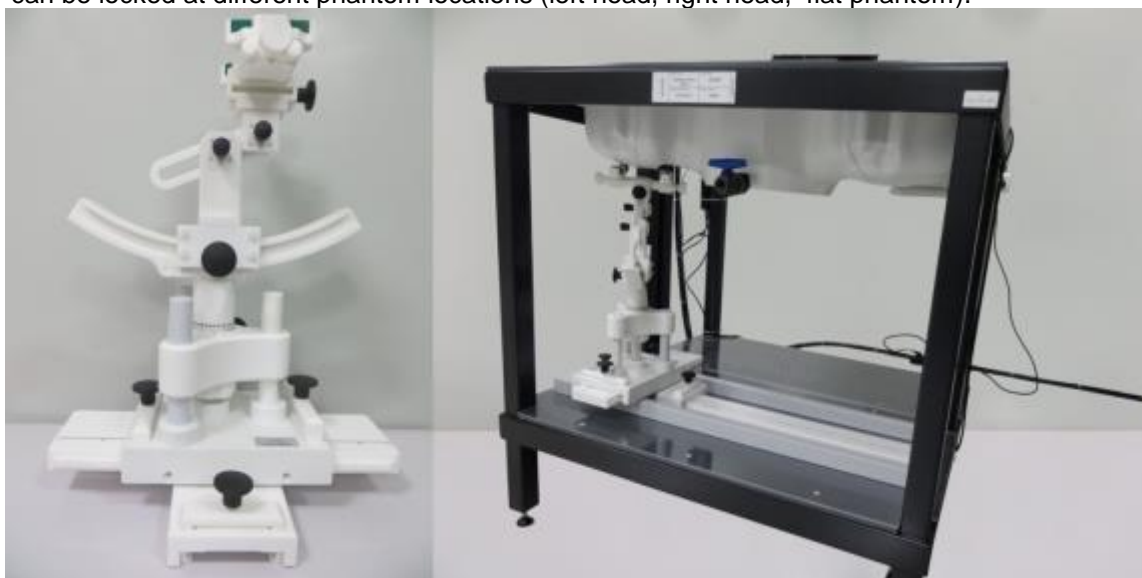
Device holder supplied by SATIMO
