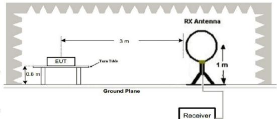
(2) Radiated Emission Test-Up Frequency 30MHz~1GHz
