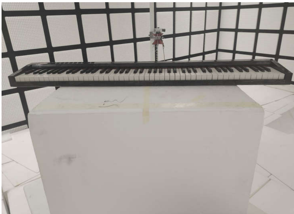
Radiated spurious emission Test Setup-2(Above 1GHz)
