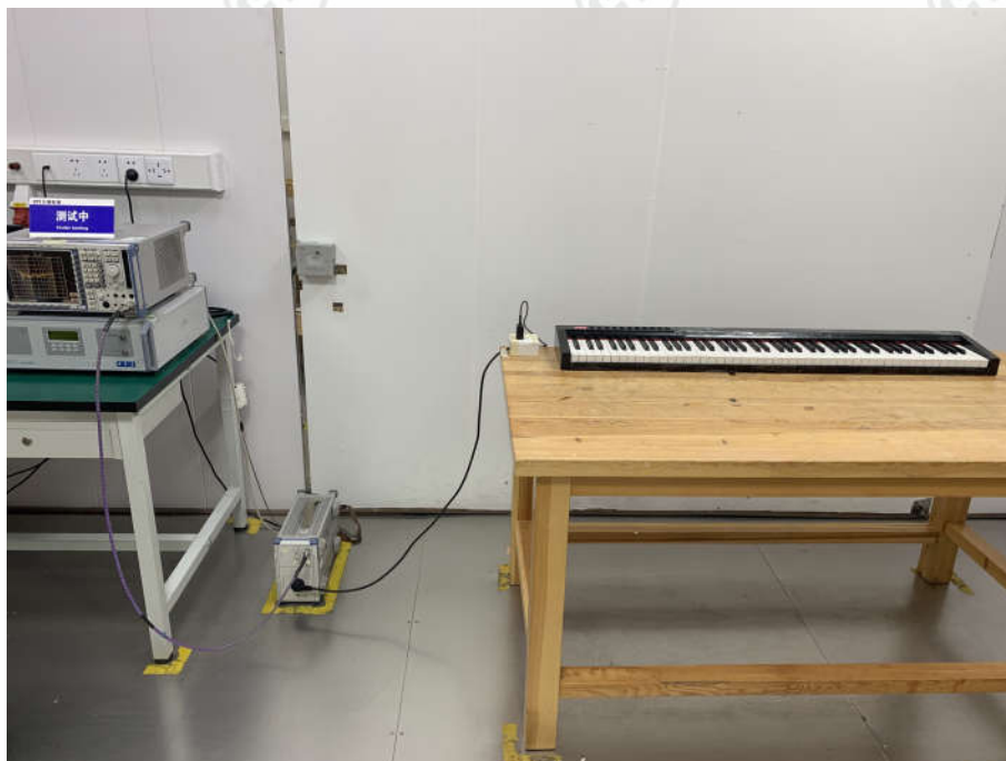
Conducted Emissions Test Setup
