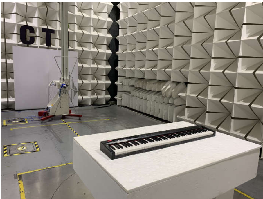
Radiated spurious emission Test Setup-1(Below 1GHz)
