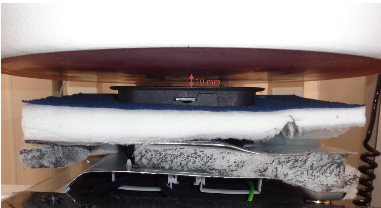
Front side of the DUT towards the phantom with 10 mm separation distance.
