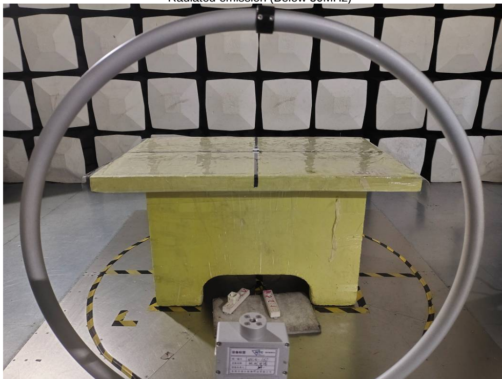
Test Photo Radiated emission (Below 30MHz)
