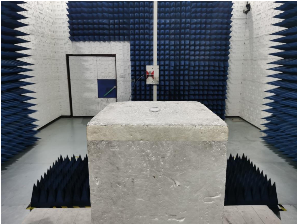
FCC RADIATED EMISSION TEST SETUP-ABOVE 1GHz
