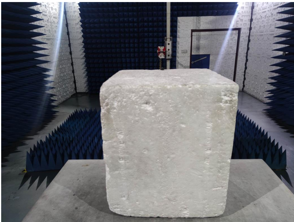
RADIATED EMISSION TEST SETUP ABOVE 1GHz
