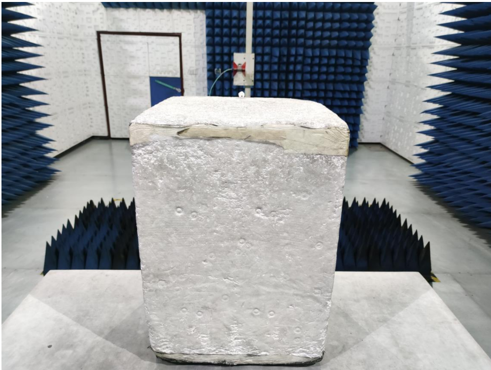
RADIATED EMISSION TEST SETUP ABOVE 1GHz
