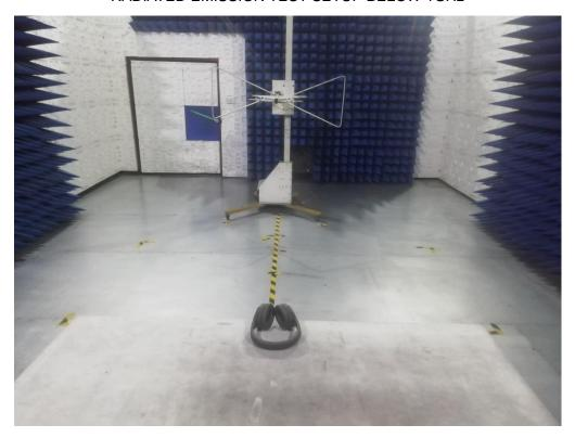
RADIATED EMISSION TEST SETUP ABOVE 1GHz
