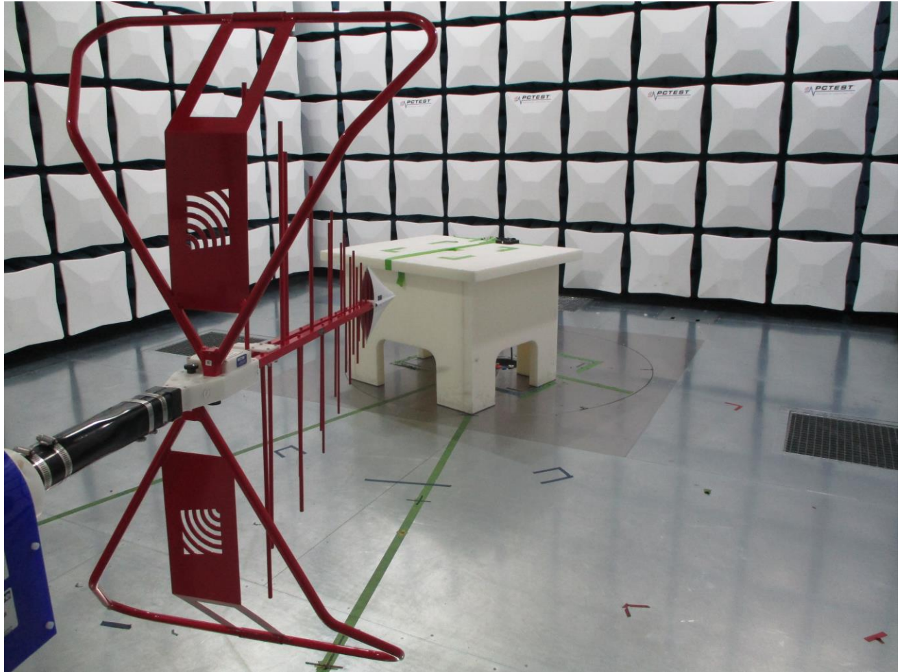
Figure 5: 30MHz-1GHz Test Setup (Front View)
