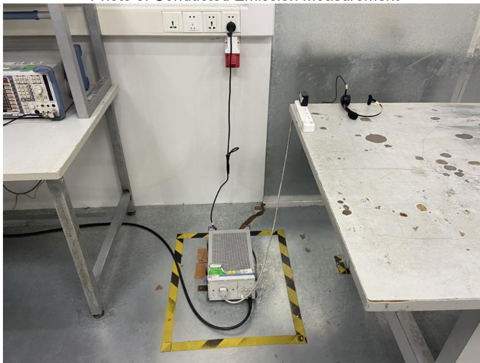
FCC ID: 2AX2I-SKBHM97 Photo of Conducted Emission Measurement
