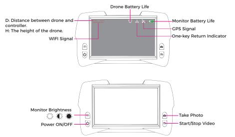
NOTE: Before using the monitor, insert a memory card to the drone to take photos and record
