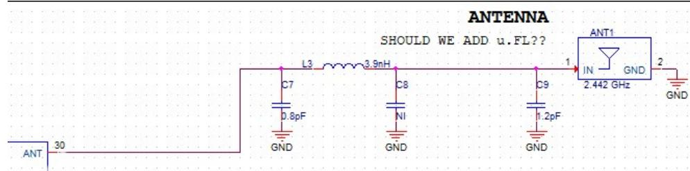
In the new revision, the GND connection to ANT1 was removed per the vendor's specification.
