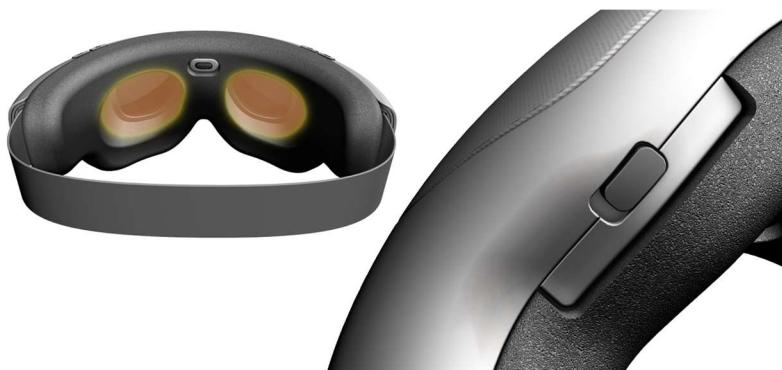
When you want to use the device, attach your headphones and slide the power switch on the bottom of the device to the ON position. The lenses will briefly illuminate amber to indicate that the device is on. This is the time to put both headphone earbuds in your ears, put the device on and prepare for the 16-minute therapy.
