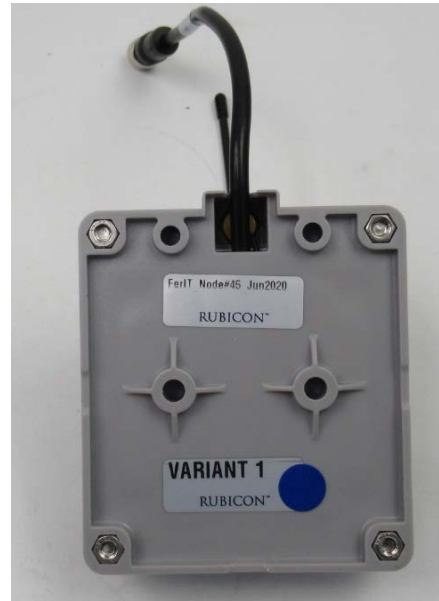
Photograph 3: Ferit Solar Node - LORA
