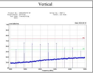
Note: Corrected Amplitude = Reading + Factor Margin = Limit- Corrected Amplitude
