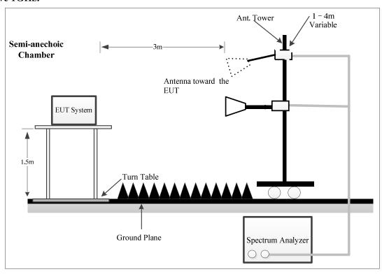
The radiated emissions were performed in the 3 meters distance, using the setup accordance with the ANSI C63.10-2013. The specification used was the FCC 15.205, 15.209, FCC 15.231 and RSS-Gen limits.
