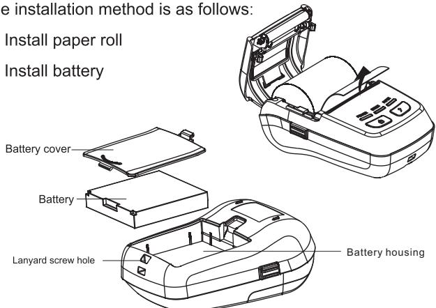
**⚠ Note:** The protective film of the battery needs to be removed before use otherwise the printer cannot be used!
