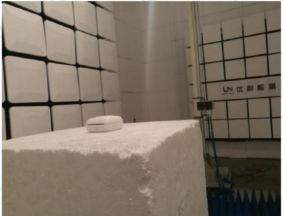
Radiated Emission (Above 1G)
