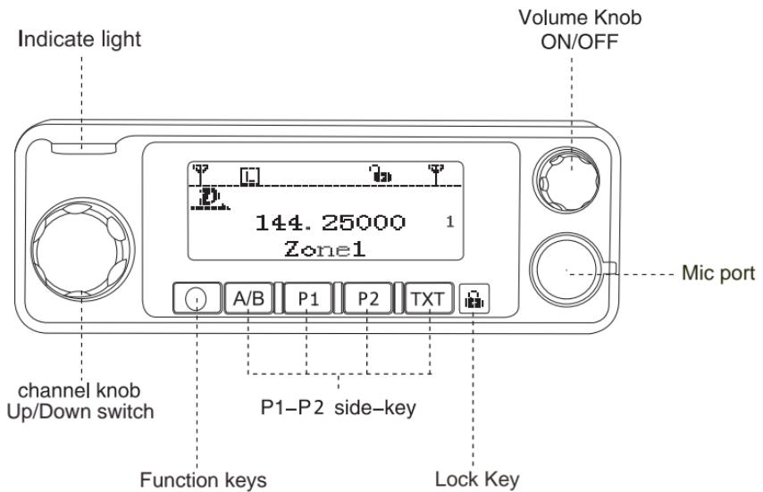
Note: Either Long press or short press of side-key1 (P1) / side-key 2 (P2) /side key 3 (A/B) / side-key 4 (TXT) can be programmed via software for the following function:
