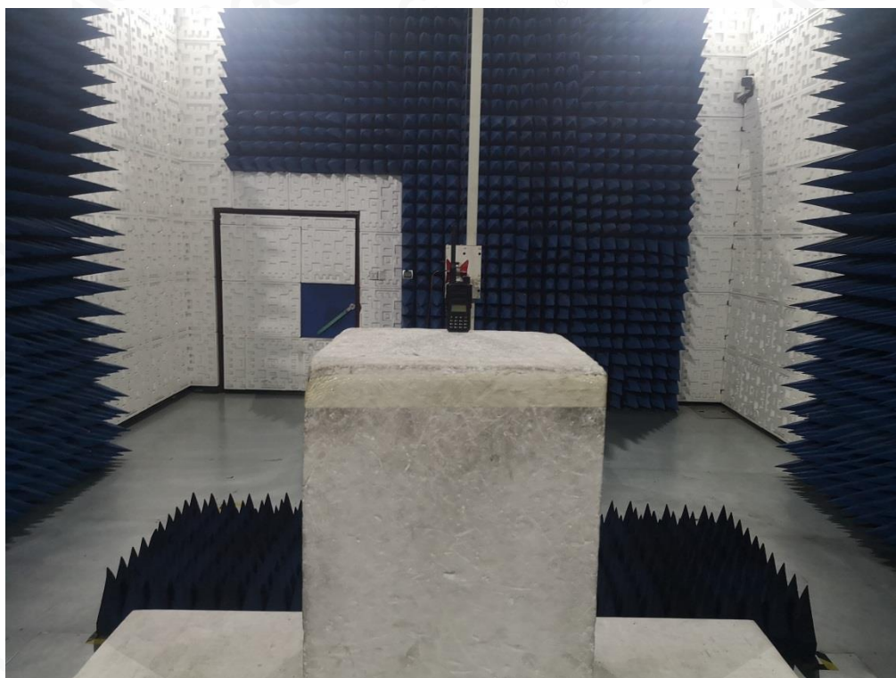
RADIATED EMISSION ABOVE 1G TEST SETUP
