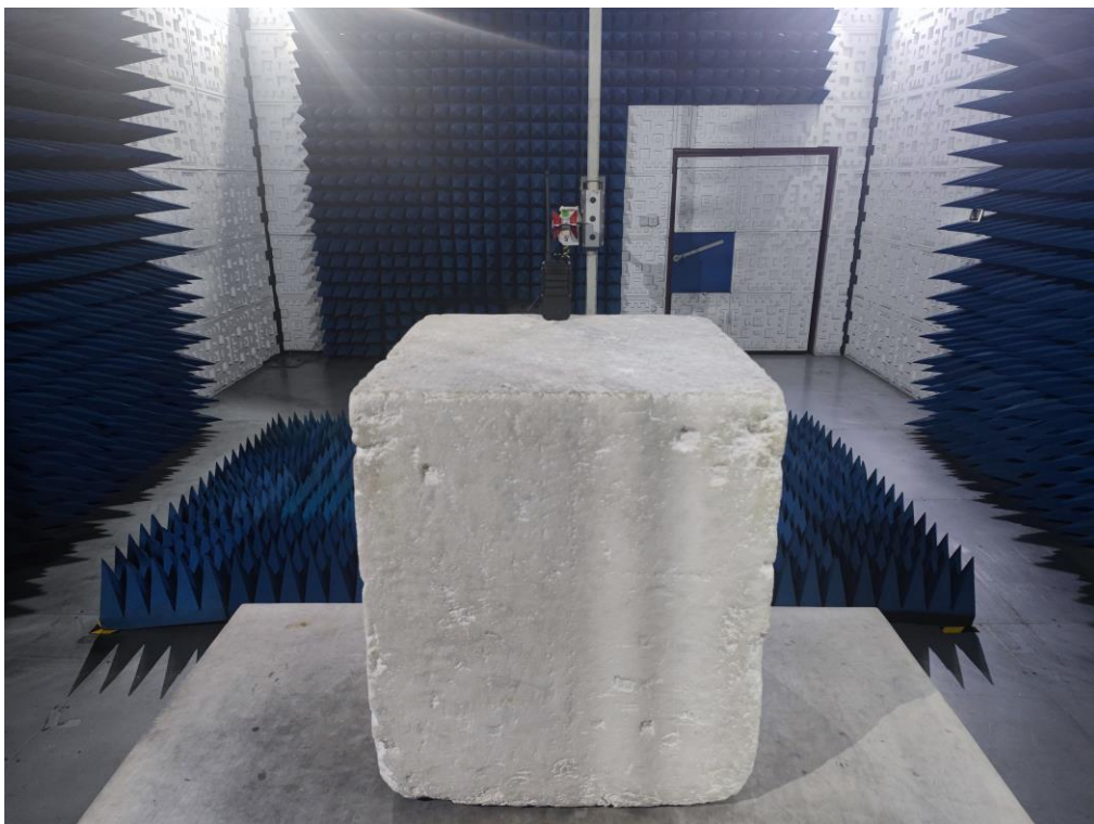
RADIATED EMISSION TEST SETUP ABOVE 1GHz
