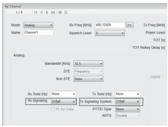
RX Signaling and Tx Signaling system choose DTMF
