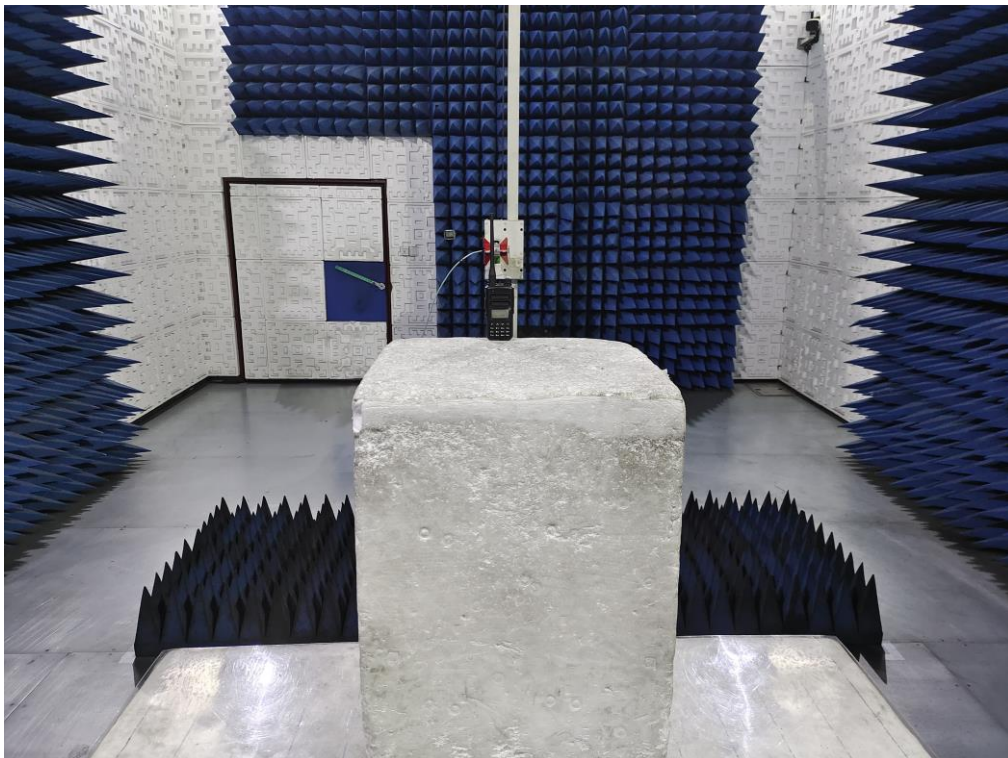
RADIATED EMISSION TEST SETUP ABOVE 1GHz
