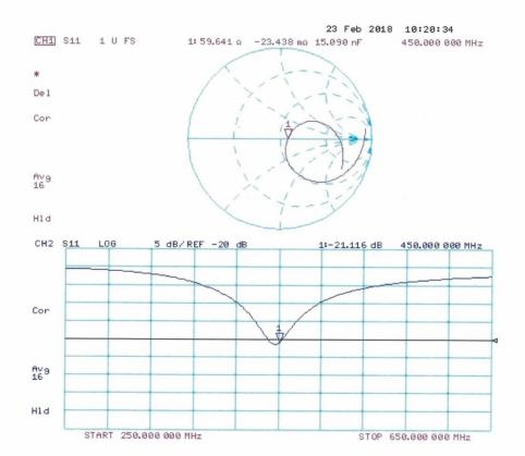
Impedance Measurement Plot for Head TSL
