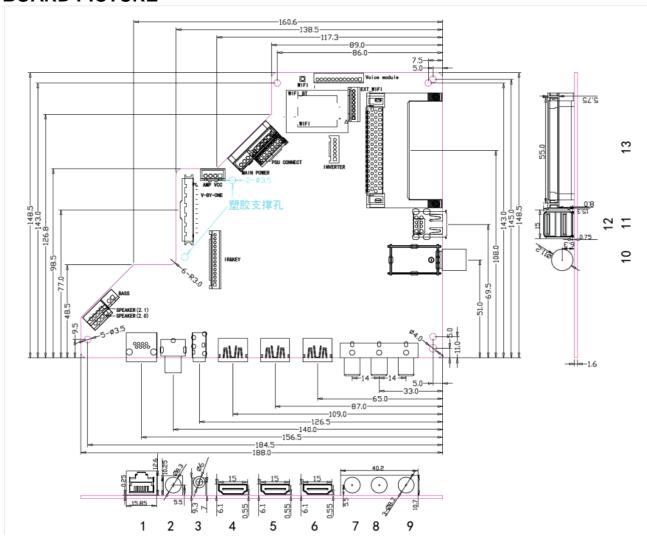
**Size:**  $188 \text{mm}(L)^* 148.5 \text{mm}(W)^* 1.6 \text{mm}(H)$
