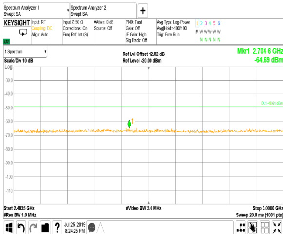
Plot 7.6.70 Band edge emission measurements in 2483.5 - 3000 MHz range at antenna chain # 7, high carrier frequency
