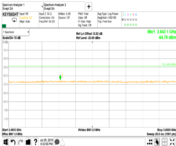
Plot 7.6.68 Band edge emission measurements in 2483.5 - 3000 MHz range at antenna chain # 6, high carrier frequency
