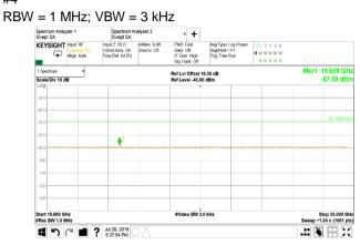
Plot 7.4.253 Spurious emission measurements in 18 - 25 GHz range at low carrier frequency CHANNEL BANDWIDTH: 5 MHz CONFIGURATION: ONE BEAM ANTENNA PORT: #5 RBW = 1 MHz; VBW = 3 MHz RBW = 1 MHz; VBW = 3 kHz Spectrum Analyzer 1 Swept SA Spectrum Analyzer 2 Swept SA Spectrum Analyzer 1 Swept SA Spectrum Analyzer 2 Swept SA • + + nout Z: 50 ( #Atten: 0 dB Source: Off
