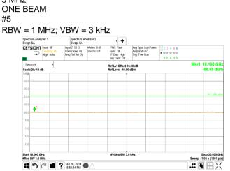
Plot 7.4.255 Spurious emission measurements in 18 - 25 GHz range at high carrier frequency CHANNEL BANDWIDTH: 5 MHz CONFIGURATION: ONE BEAM ANTENNA PORT: #5 RBW = 1 MHz; VBW = 3 MHz
