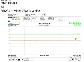
Plot 7.4.269 Spurious emission measurements in 18 - 25 GHz range at mid carrier frequency CHANNEL BANDWIDTH: 10 MHz CONFIGURATION: ONE BEAM ANTENNA PORT: #2 RBW = 1 MHz; VBW = 3 MHz
