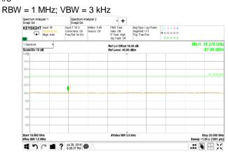
Plot 7.4.259 Spurious emission measurements in 18 - 25 GHz range at low carrier frequency CHANNEL BANDWIDTH: 5 MHz **CONFIGURATION:** ONE BEAM ANTENNA PORT: #7 RBW = 1 MHz; VBW = 3 MHz RBW = 1 MHz; VBW = 3 kHz Spectrum Analyzer 1 Swept SA KEYSIGHT Input: RF Coupling DC Align: Auto Spectrum Analyzer 2 Swept SA Spectrum Analyzer 1 Swept SA Spectrum Analyzer 2 Swept SA • + + input Z: 50 C #Atten: 0 dB Source: Off Avg Type: Log-Avg(Hold.>1/1 Trig: Free Run
