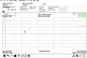
Plot 7.4.265 Spurious emission measurements in 18 - 25 GHz range at low carrier frequency CHANNEL BANDWIDTH: 10 MHz CONFIGURATION: ONE BEAM ANTENNA PORT: #1 RBW = 1 MHz; VBW = 3 MHz
