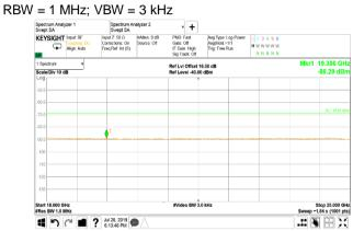
Plot 7.4.261 Spurious emission measurements in 18 - 25 GHz range at high carrier frequency
