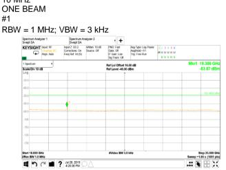
Plot 7.4.267 Spurious emission measurements in 18 - 25 GHz range at high carrier frequency CHANNEL BANDWIDTH: 10 MHz CONFIGURATION: ONE BEAM ANTENNA PORT: #1 RBW = 1 MHz; VBW = 3 MHz
