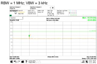
Plot 7.4.243 Spurious emission measurements in 18 - 25 GHz range at high carrier frequencyCHANNEL BANDWIDTH:5 MHzCONFIGURATION:ONE BEAMANTENNA PORT:#1RBW = 1 MHz; VBW = 3 MHzRBW = 1 MHz; VBW = 3 kHz
