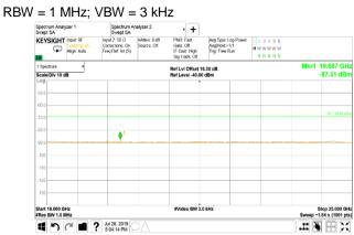
Plot 7.4.273 Spurious emission measurements in 18 - 25 GHz range at high carrier frequency CHANNEL BANDWIDTH: 10 MHz **CONFIGURATION:** ONE BEAM ANTENNA PORT: #3 RBW = 1 MHz; VBW = 3 MHz
