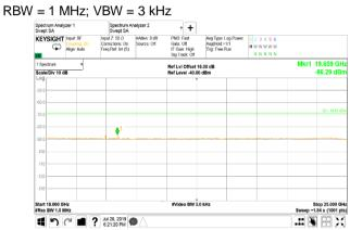
Plot 7.4.263 Spurious emission measurements in 18 - 25 GHz range at mid carrier frequencyCHANNEL BANDWIDTH:5 MHzCONFIGURATION:ONE BEAMANTENNA PORT:#8RBW = 1 MHz; VBW = 3 MHzRBW = 1 MHz; VBW = 3 kHz
