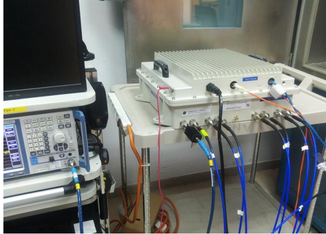
Photograph No.4 Setup for OBW measurements
