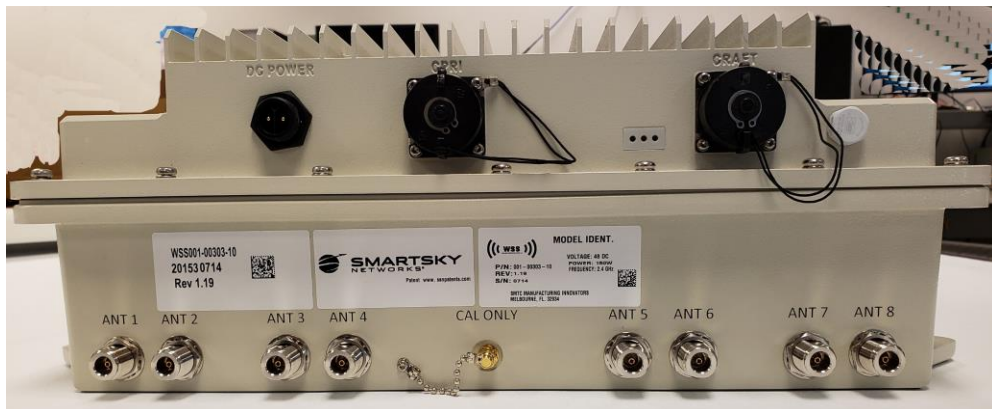
Figure 2 – RRH Front View
