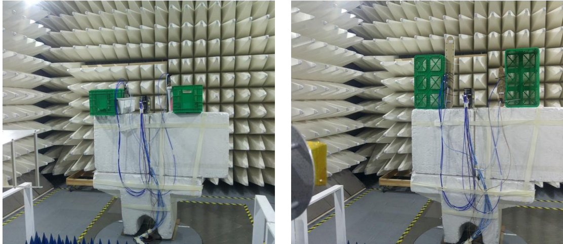
Photograph No.3 Setup for spurious emission field strength measurements in the anechoic chamber above 1000 MHz range
