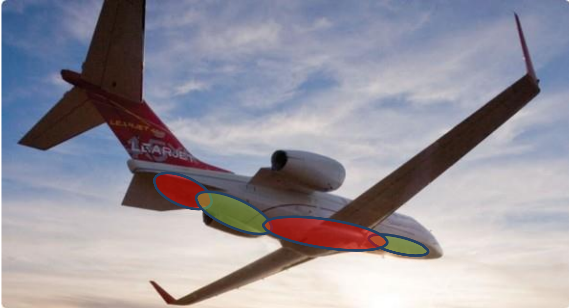
Figure 3.5.1-2 Antenna Location Preferences – Learjet 45 Example (green) and keep-out areas (red) for Aircraft with Ventral Fins
