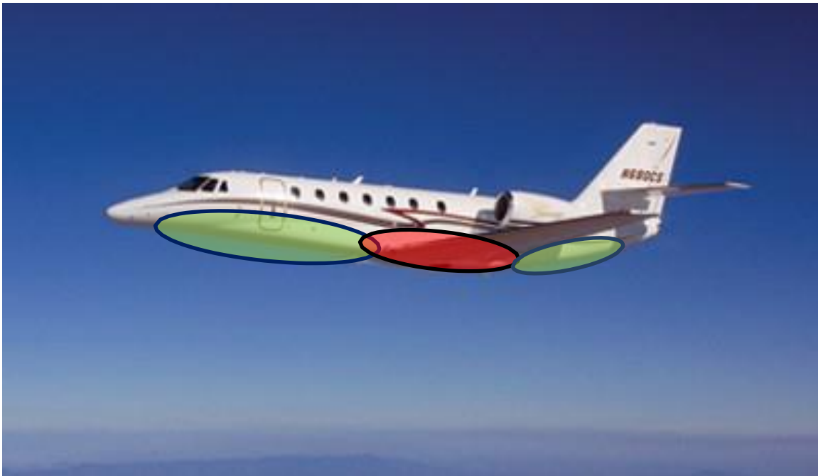
Figure 3.5.1-3 Antenna Location Preferences – Citation Sovereign Example (green) and keep-out areas (red) for Aircraft without Ventral Fins
