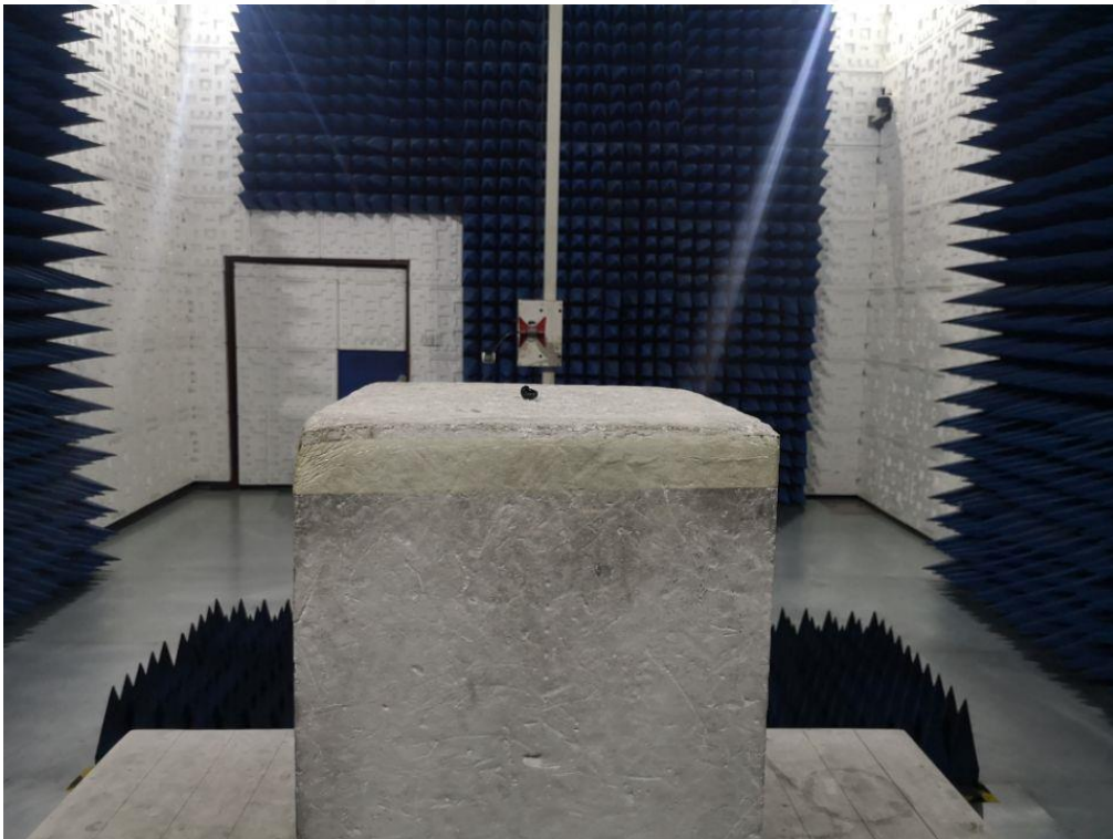
RADIATED EMISSION TEST SETUP ABOVE 1GHZ
