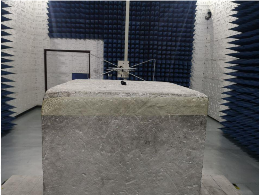
RADIATED EMISSION TEST SETUP ABOVE 1GHZ
