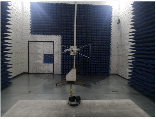
RADIATED EMISSION TEST SETUP ABOVE 1GHz
