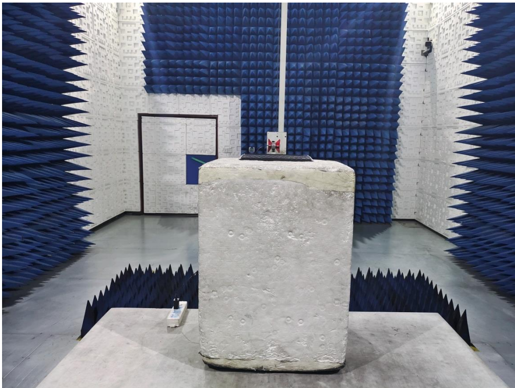
RADIATED EMISSION TEST SETUP ABOVE 1GHz
