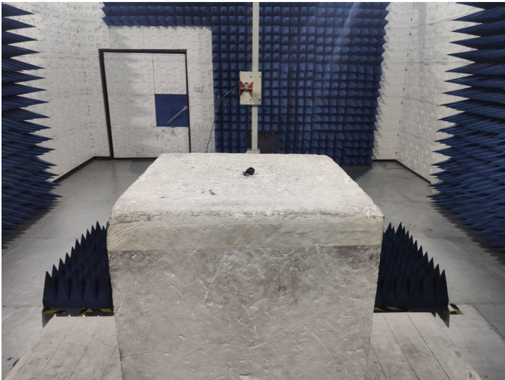
RADIATED EMISSION TEST SETUP ABOVE 1GHz
