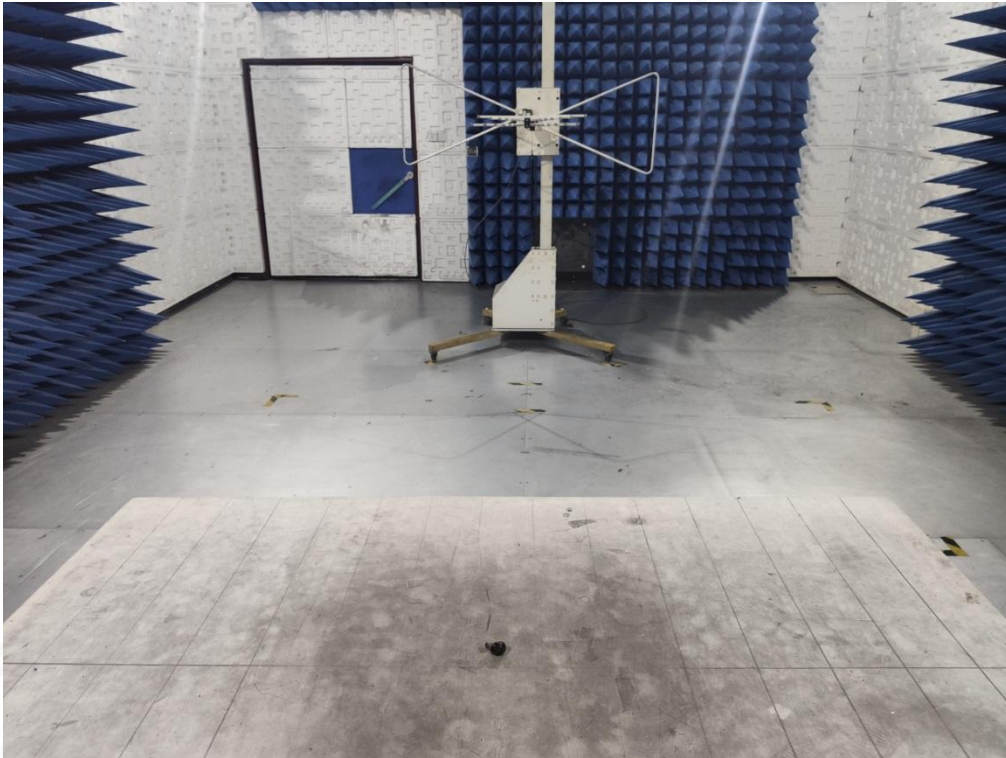
RADIATED EMISSION TEST SETUP ABOVE 1GHz
