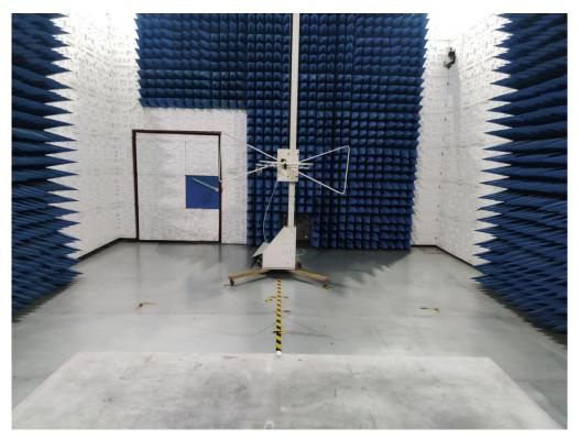
RADIATED EMISSION TEST SETUP ABOVE 1GHZ
