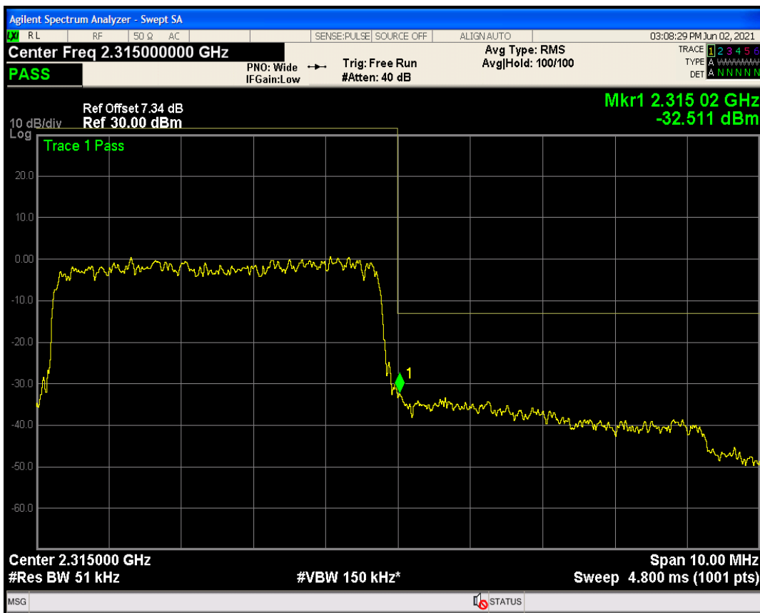
Band40a QAM16 BW=5MHz Channel=38775 RB Size=25 Position=#0
