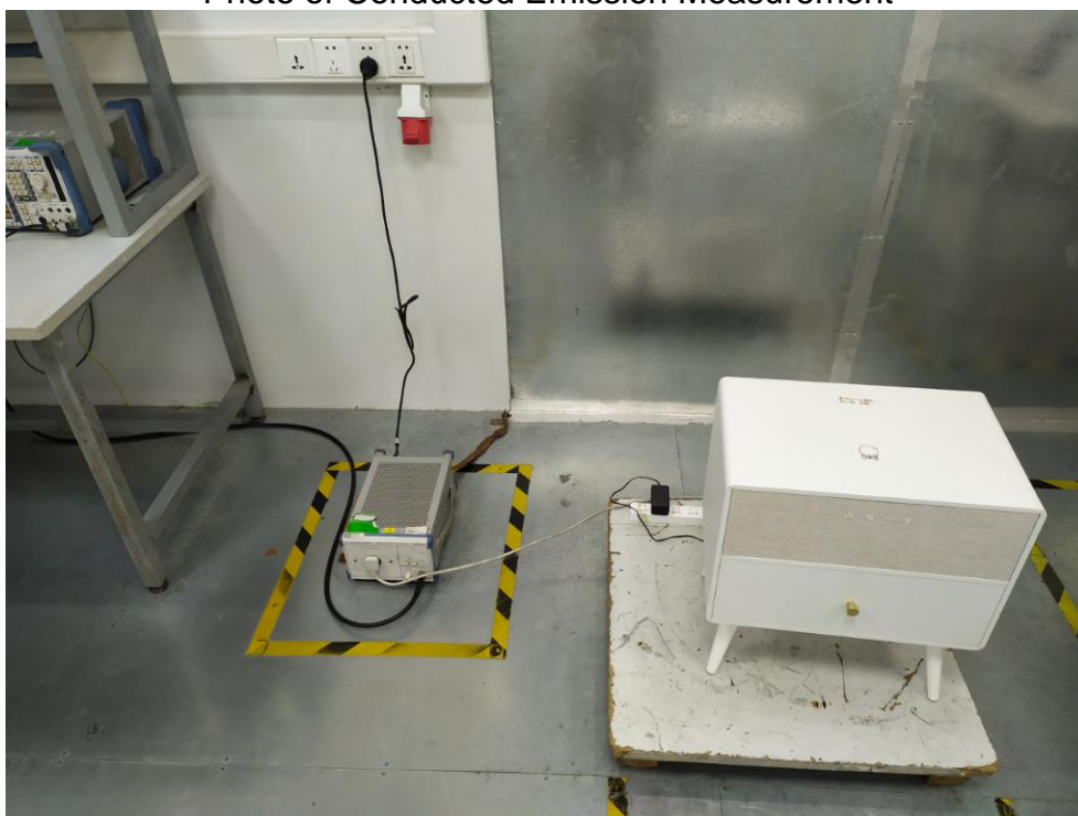
FCC ID: 2AWWQ-KBBM1115 Photo of Conducted Emission Measurement
