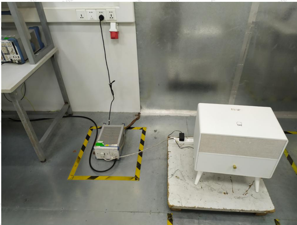
Photo of Conducted Emission Measurement
