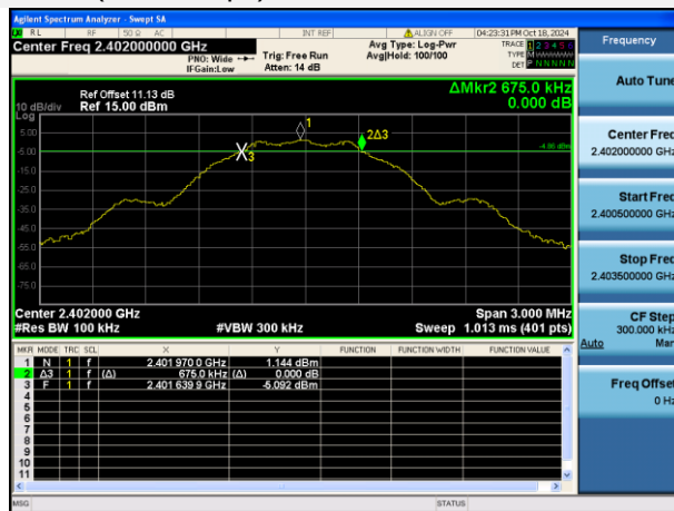
GFSK (BLE 1Mbps) LOW CHANNEL
