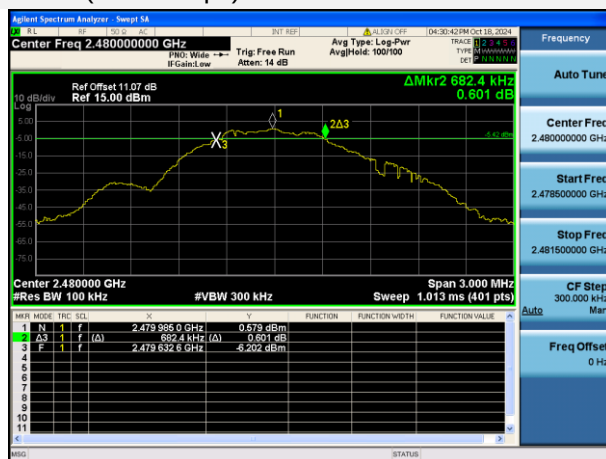
GFSK (BLE 1Mbps) HIGH CHANNEL
