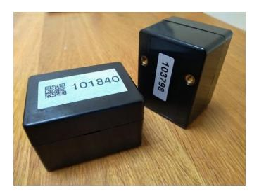
Sensize Dot DT1.4L is an ultra-long battery life, low-cost tracker with Bluetooth technology. The size and shape of its enclosure makes it particularly easy to secure onto plastic pallets and containers. Part of Sensize's Parent/Child tracking architecture, Dot v1.4L, when used in a system with Sensize Access Points, Cellular Trackers, Scanners and Gateways, offers a low cost, highly effective way to track and monitor assets such as pallets, roll cages and reusable plastic crates.
