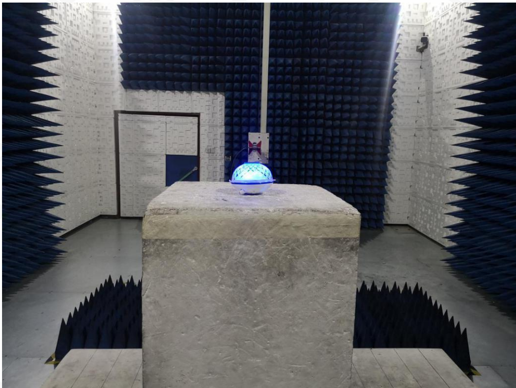
RADIATED EMISSION TEST SETUP ABOVE 1GHZ
