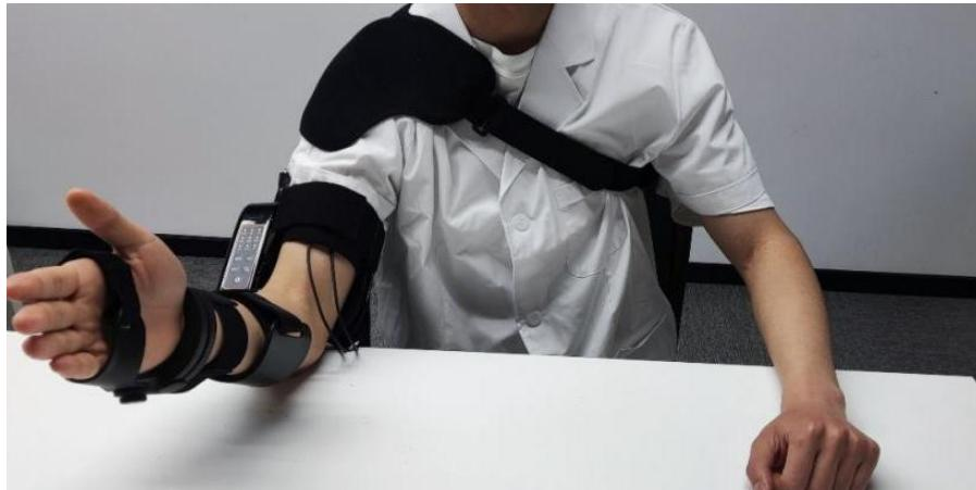
After wearing the shoulder strap, connect the exoskeleton to the shoulder strap through three straps.
