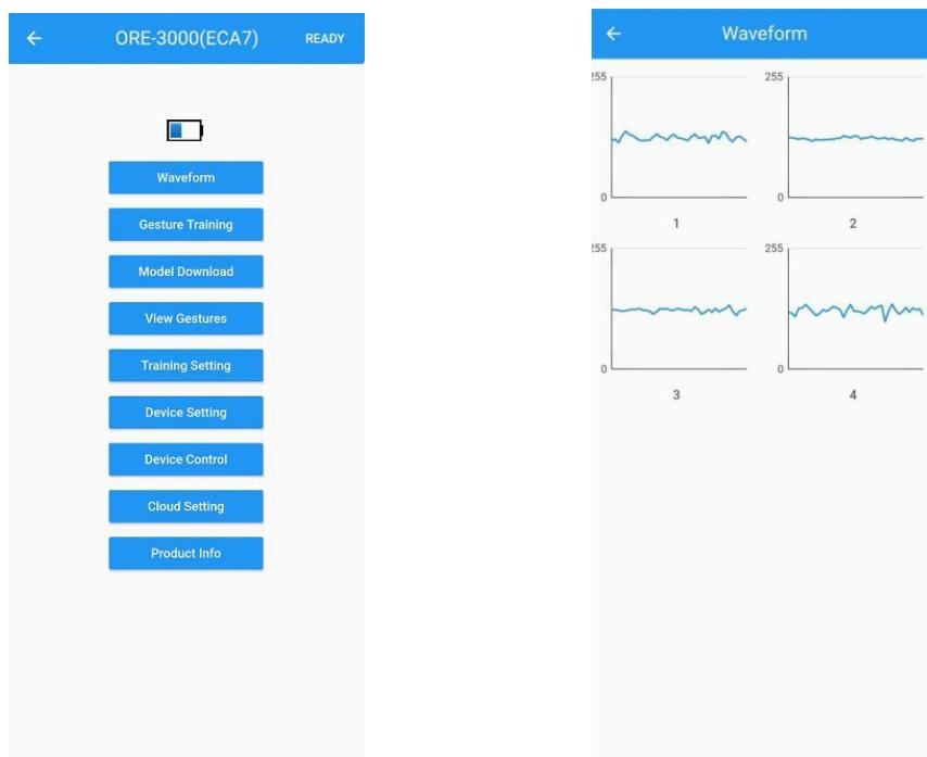
(1) This function displays real-time waveforms of various EMG signals, making it easy for users to check data transmission, check sensor connection quality, detect signal interference, etc.
