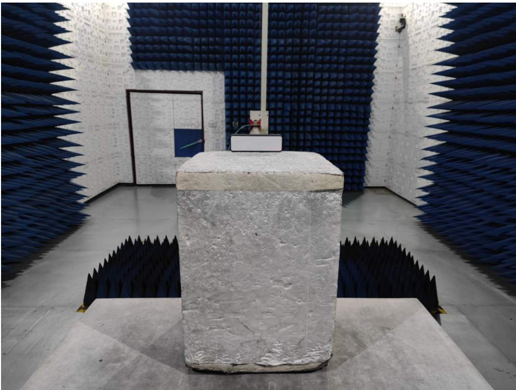
RADIATED EMISSION TEST SETUP ABOVE 1GHZ
