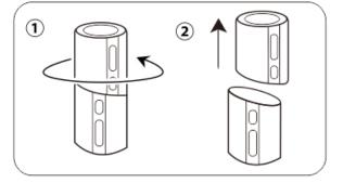
Rotate the top part to the right and leave the bottom part at an Angle of picture ① position to separate the two parts like the picture ②.
