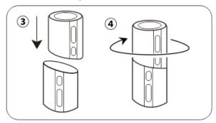
Put an angle of the picture ③ position, connect the two parts together and rotate the top part to the left unit it locks like the picture ④.
