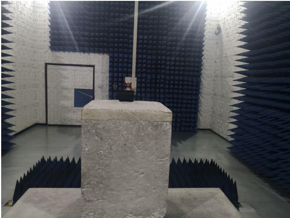
RADIATED EMISSION TEST SETUP ABOVE 1GHz
