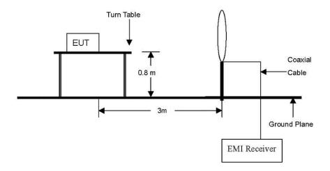
The diagram below shows the test setup that is utilized to make the measurements for emission from 30 Mb to 1 GHz emissions.
