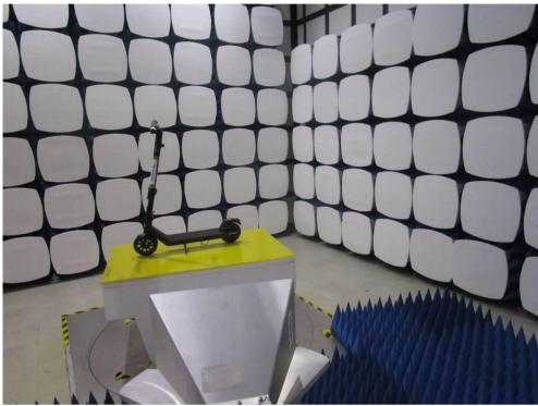
1.2 Radiated spurious Emissions Test Setup
